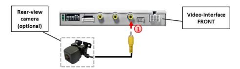
1 Connect the video-RCA of the after-market rear-view camera to the female RCA port of the video-interface which is labeled as CAM.
