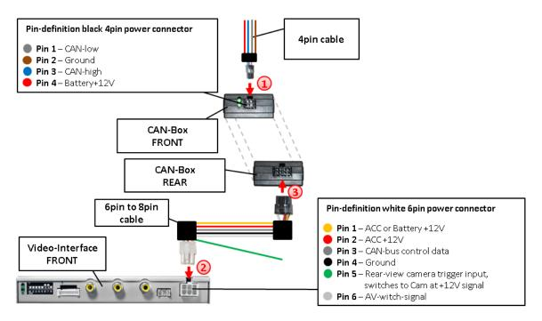
1 Connect CAN-bus and power at the rear of the factory monitor, otherwise no interface function! The connector can be different to the pictured connector.
