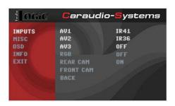
**Note:** The IR-control channel AV1 is preset to RC-Code 41 compatible DVB-T tuners and AV2 is preset to RC-Code 36 for the usbLiNK2.
