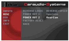
On some vehicles the reverse light signal doesn't exist on the CAN-bus. Connect the white wire of harness V4C-MBN45 to reverse light signal (+12V of reverse light) if the v.LOGiC doesn't switch to the rear-view camera automatically after the described OSD-setup (see next chapter).
