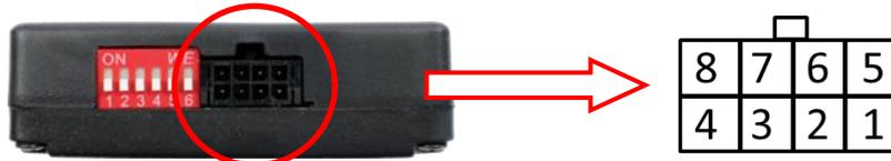
Pin-assignment male 8pin connector of TV-500
