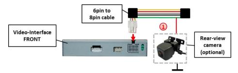
1 In addition power supply of +12V (500mA max.) of the After-Market Rear View Camera can be realised by the green wire of of 6Pin to 8pin cable
