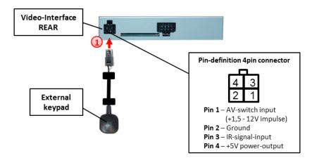
Connect 4pin female Microfit connector of external keypad to male 4pin Microfit connector of video interface
