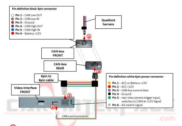
Connect black female 4pin Micro-Fit connector of the 4pin cable to the male 4pin Micro-Fit connector of the CAN-box.
