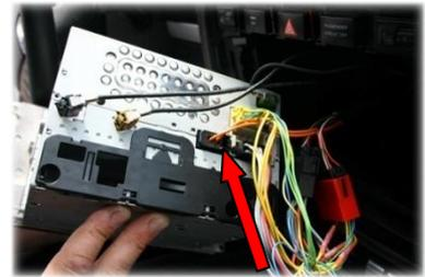
Connect black wire to ground and red wire to permanent +12V. Isolate blue wire.
