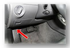
2. Connect the TV302HM interface to the OBD socket for about 15 seconds in order to activate the function.
