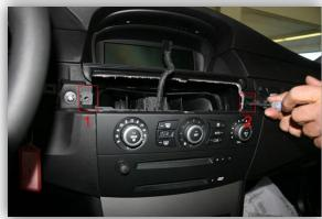
Remove climate control panel. Remove CD/DVD drive trim. Trim is fixed by 2 screws on the upper side and plugged to the lower trim. Remove the lower trim (plugged too).
