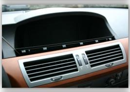
Flip down the board monitor. *NOTE*: The OEM screen gets stuck with its connector at the upper side of the cockpit. Insert a hard plastic sheet like a credit card to prevent cockpit from taking damage.
