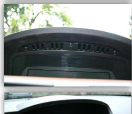
Remove cover grill (only plugged). Place soft towel beneath the board monitor to avoid scratches
