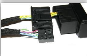
Insert the completed black connector into CAN interface harness TV-BM65.
