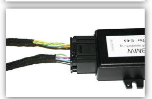
Connect 12-pin insert from CAN interface harness TV-BM65 into black connector from vehicle harness.
