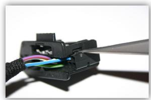
Insert 12-pin insert into black connector of the CAN interface harness TV-BM65.
