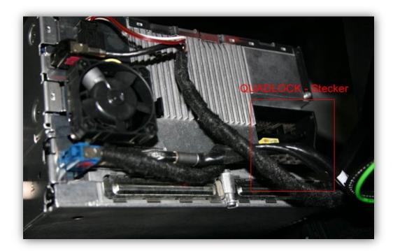
The Quadlock connector includes different chambers. If present, remove the white, black and the optical inserts, from the vehicle harness' Quadlock connector. Plug the vehicle harness' Quadlock connector into the male Quadlock connector of the CAN interface harness TV-BM01
