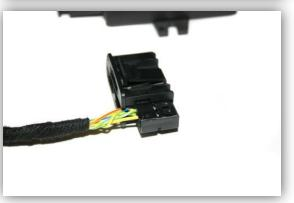
Insert completed connector into the plug on the backside of the board monitor.
