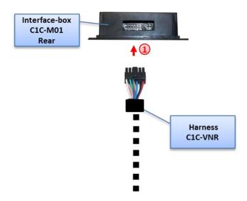
1 Plug harness C1C-VNR into 12pin Molex of Interface-Box C1C-M01.
