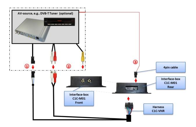
Using the respective STA-xxx IR-control cable, interconnect the blue female 3pin AMP connector of harness C1C-VNR and the IR-port of the AV-source.
