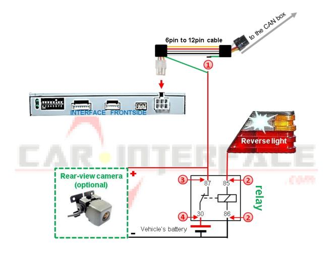
Out the green cable of the 6pin to 12pin cable close to the black 12pin connector and isolate the shorter end of the green cable near to the 12pin connector (CAN-box side).
