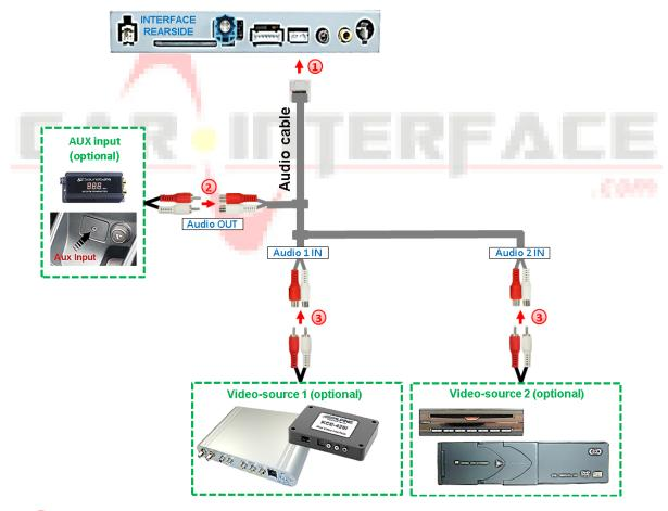
Connect the audio cable's female 7pin connector to the male 7pin connector of the video-interface.
