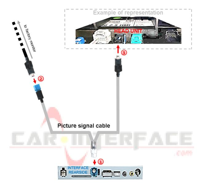
Connect the enclosed picture signal cable's female white coloured HSD connector to the male waterblue coloured HSD connector of the video interface.
