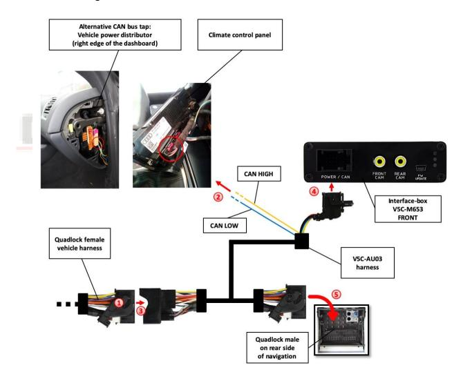
Remove the female Quadlock connector of the vehicle harness from the rear of the navigation computer.
