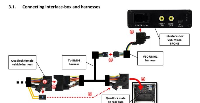
Remove the female Quadlock connector of the vehicle harness from the rear of the navigation computer.
