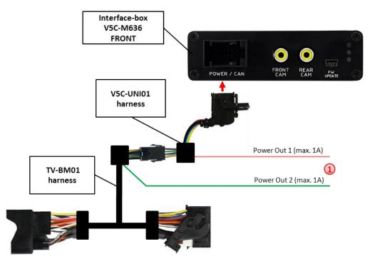
You can configure the both +12V trigger outputs separately. The pink wire is POWER OUT 1 and the green wire is POWER OUT 2.
