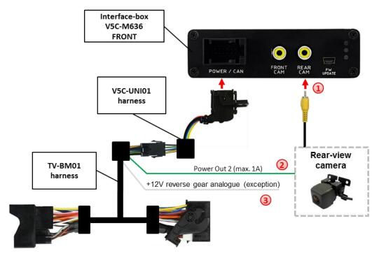
Connect the video RCA of the after-market rear-view camera to the female RCA connector "REAR CAM" of the interface box V5C-M631.
