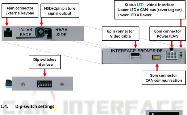
Some settings must be selected by the dip-switches on the video-interface. Dip position down is ON and position up is OFF.
