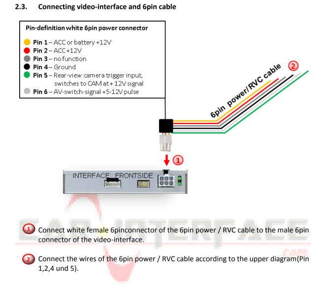
**Note:** Check the LEDs on video-interface after reconnecting the battery, one has to be on.
