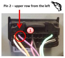
① Cut the cable at pin 2 of the upper row from the left side and isolate both ends.
