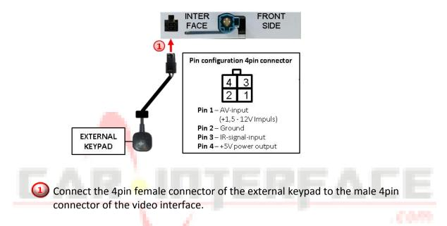
**Note:** Regardless if it'll be used or not, the external keypad should always be connected! In case of non-using, it should be invisibly hidden together with the video interface.
