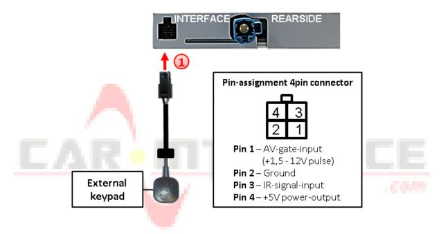
Connect the 4pin female connector of the external keypad to the male 4pin connector of the video interface.
