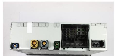
3. Connect the black wire of the cable kit to ground and the red wire to 12V plus. The corresponding control cable (e.g. for DVD device) is not supported.
