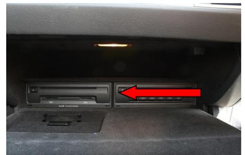
2. Disconnect the original Quadlock-connector from the device. Connect the green Fakra-plug (Video-Line) to the Navigation unit. Remove one of the two optical cables from the original Quadlock-connector and connect it to the enclosed LWL-connector. Connect the second optical cable to the original Quadlock-connector. Pay attention to the directional arrows as shown in the picture on the right.
