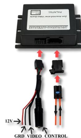
4. Connect the three Cinch sockets of the interface to the video source using a Video / Audio Cinch cable (not included).
