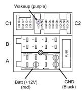
The pinout of certain Comand head units can differ from the above drawing. If the GND and +12V pin of your Head Unit can be found in the position as indicated in the following picture, then the wakeup wire should be connected to a different pin.
