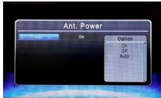
*Important note: If an amplified antenna has not been connected to the tuner before the tuner's 12V power connection, the necessary +12V power supply won't succeed! To guarantee the necessary phantom power supply, either the connection of the antenna has to be done as the first step, or alternative performing the system's power reset would be a solution.*
