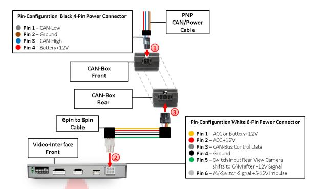
1 Connect the black female 8pin Micro-Fit connector of the PNP Power/CAN harness to the male 8pin Micro-Fit connector of the CAN-box.
