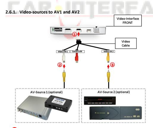
1 Connect the video cable's female 6pin connector to the video interface's male 6pin connector.
