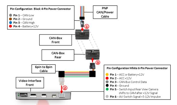
1 Connect the black female 8pin Micro-Fit connector of the PNP Power/CAN harness to the male 8pin Micro-Fit connector of the CAN-box.
