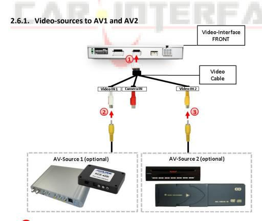
1 Connect the video cable's female 6pin connector to the video interface's male 6pin connector.
