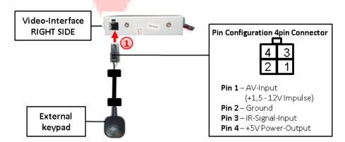
1 Connect the female 4pin connector of the keypad to the male 4pin connector of the video-interface.
