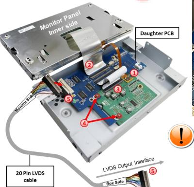
If there is a housing screw at the position marked above during reassembly, it must not reach into the interior of the housing, otherwise, as shown in the picture, the LVDS connector may be damaged when screwed in!
