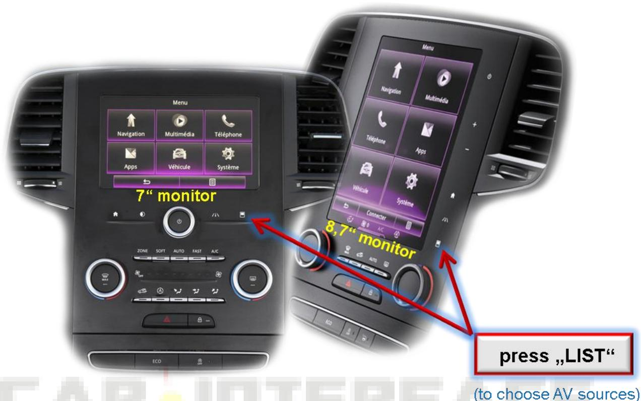
Pressing the “LIST” button switches the input from the factory video to the inserted video sources. If all inputs are activated by dip switch settings, the order is the following:
