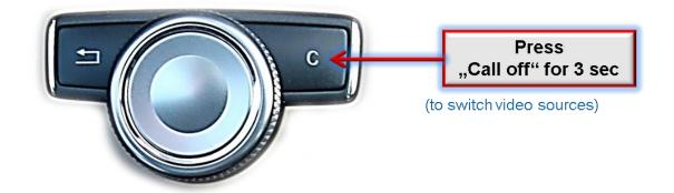
**Long press C button** (3 sec.) beside knob in centre console to switch the video source. Each repetition will switch to the next enabled input. If all inputs are enabled the order is:
