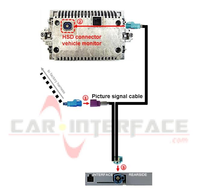
Remove the blue female 4pin HSD connector from the rearside of the factory monitor and connect it to the aubergine colored male 4pin HSD connector of the picture signal cable.
