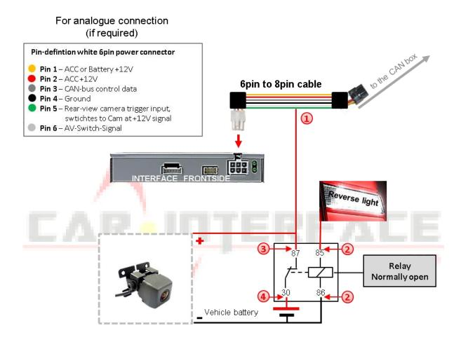
Connect the green wire of the 6pin to 8pin cable to the output connector (87) of the relay.
