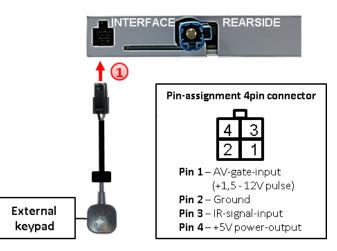
Connect the female 4pin connector of the keypad to the male 4pin connector of the video-interface.
