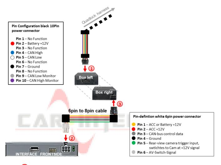
Connect theblack female 10pin connector of the Quadlock harness to the male 10pin connector of the CAN-box.
