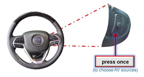
A press of the volume button on the right rear side of the steering wheel switches the input from factory mode to the inserted video sources. If -by dip switch setting- all inputs are enabled, the order will be the following:
