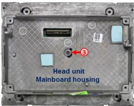
3 Turn out the Torx screw (T10) at the middle of the head unit's mainboard housing and carefully put the housing aside to set free the monitor panel with its kopper coulored picture ribbon cable
