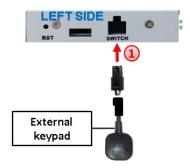
Onnect the external keypad's female 4pin connector to the video-interface's male 4pin connector.
