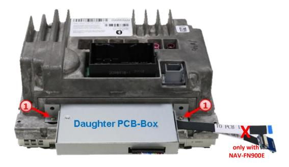
Screw in the daughter PCB box at the rearside of the head-unit by using the enclosed screws
