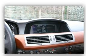
Remove 3 TORX screws at the OEM screen.
