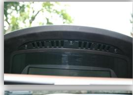
Remove cover grill (only plugged). Place soft towel beneath the navigation monitor to avoid scratches
