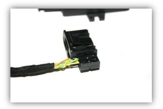
Insert completed connector into the plug on the backside of the navigation monitor. Connect 8pin Molex connector of TV-BM65 to CAN-box TV-401.
