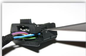
Insert 12-pin insert into black connector of the harness TV-BM65.
