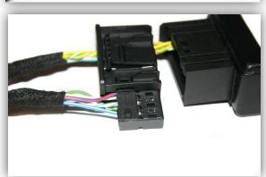
Insert the completed black connector into harness TV-BM65.
