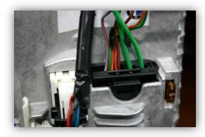
Remove 12-pin insert from black vehicle harness connector.
