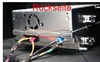
Unplug the insert from the 20-pin socket.
