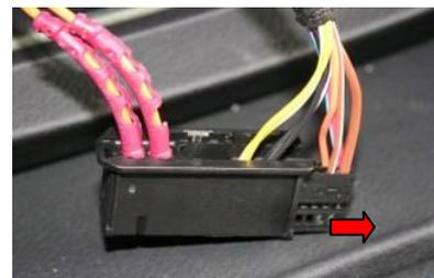
Loosen Pin 1 (yellow / white cable, CAN HIGH) and Pin 11 (yellow cable, CAN LOW) from the 20-pin socket and, as shown in the right-hand-side illustration, pin it in the included 3-pin socket.
