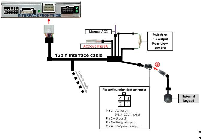
Connect the female 4pin connector of the keypad to the male 4pin connector of the 12pin interface cable.
