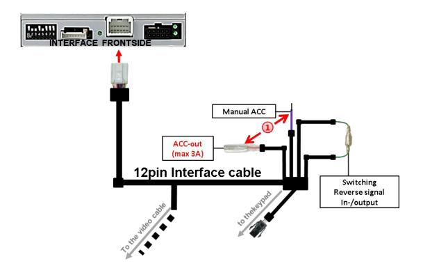
If, after connecting the PNP harness, no interface LED lightens up while the ignition is turned on, the single red wire ACC-out (max 3A) and the purple coloured wire Manual ACC of the 12pin interface cable both have to be connected additionately to S-contact terminal 86s +12V (e.g. glove compartment illumination).
