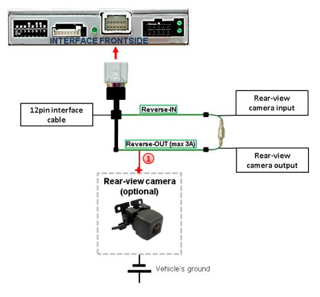
Additionally, the +12V (max. 3A) power supply for the rear-view camera can be taken from the green wire of the 12pin interface cable.
