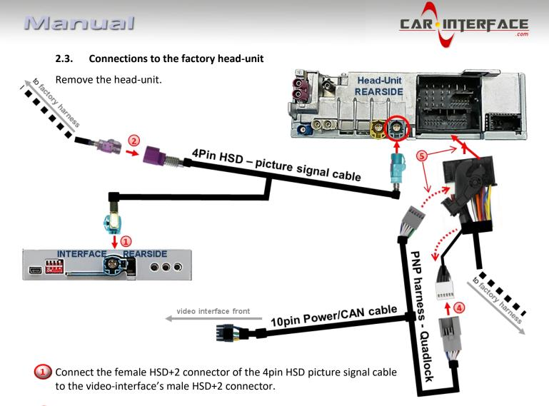
Disconnect the female 4pin HSD connector of the vehicle harness from the rear of the head-unit and connect it to the male 4pin HSD connector of the 4pin HSD picture signal cable.
