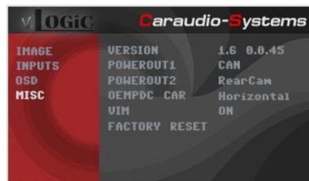
**3** On some vehicles the reverse light signal doesn’t exist on the CAN-bus. Connect the white wire of harness TV-BM01 to reverse light signal (+12V of reverse light) if the system doesn’t switch to the rear-view camera automatically after the described OSD-setup (see next chapter).
