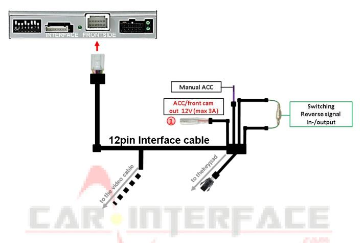
1 The red power supply output ACC/front cam out 12V (max 3A) can be used to power an external source and has a different assignment, depending on the position of dip switch 1 (of 8 dips):
