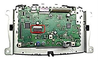
Disconnect the ribbon cable from the mainboard's ribbon cable base, as shown above.
