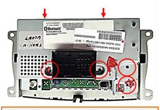
Turn out the screws shown above, to remove the head unit housing's rear cover.
