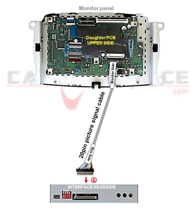
Connect the female 20pin connector "Box Side" of the daughter PCB's pre-connected 20pin picture signal cable to the video interface's male 20pin connector.
