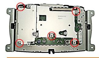
Turn out the 5 screws shown above to remove the metal cover from the screen.
