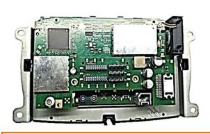
Carefully separate the original PCB from the system. Make sure not to damage the connector.
