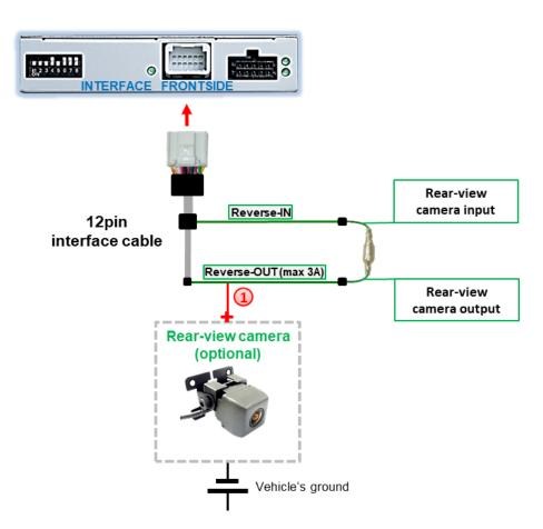
1 The 12 V power supply for the rear-view camera (max 3A) has to be taken from the green wire of the 20pin cable to avoid an unnecessary permanent power supply to the camera electronic.
