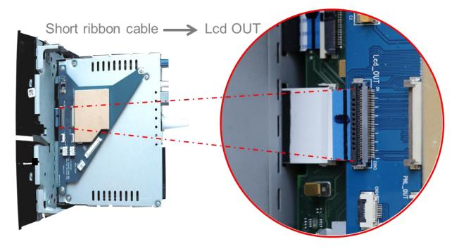
Onnect the daughter PCB's pre-assembeled 40pin ribbon cable to the previously become free ribbon cable base of the head-unit mainboard. (heed the following warning notes!).
