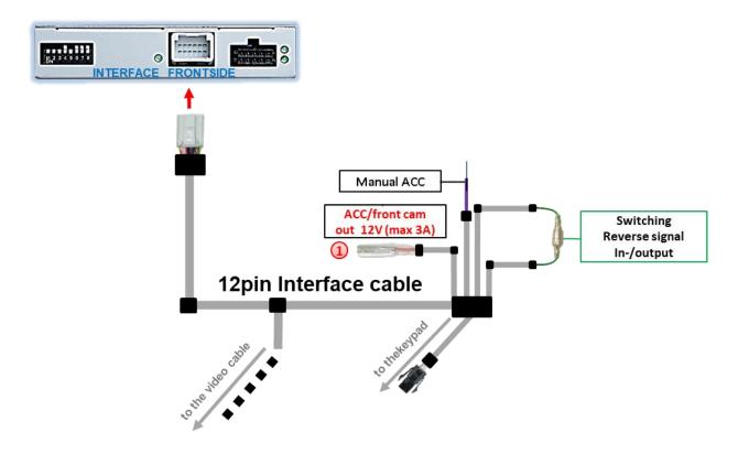
The red power supply output ACC/front cam out 12V (max 3A) can be used to power an external source and has a different assignment depending on the position of dip switch 1 (of the black 8 dips):
