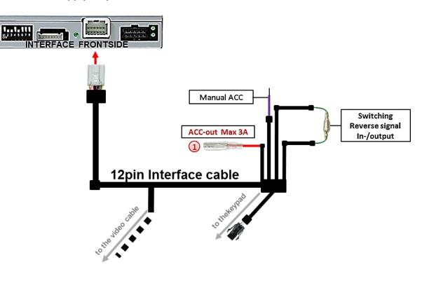
(1) The red power supply output ACC-out Max 3A can be used to power an external source (max 3A).
