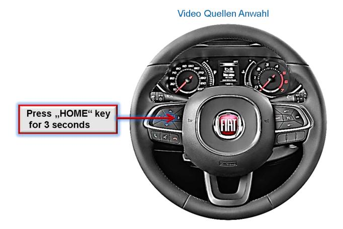
To switch the interface's activated video sources, the factory infotainment buttons can be used.
