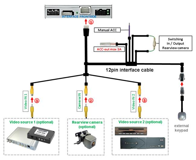
Connect the 12pin interface cable's female 12pin connector to the male 12pin connector of the video-interface.
