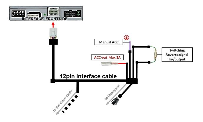
Connect the purple coloured wire Manual ACC of the 12pin interface cable to +12V ACC power supply
