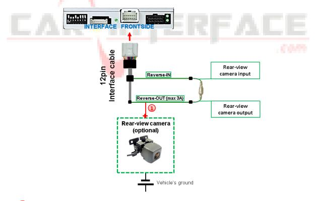
Additionally, the +12V (max. 3A) power supply for the rear-view camera can be taken from the green wire of the 12pin interface cable.
