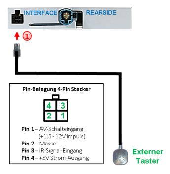
Onnect the keypad's female 4pin connector to the video-interface's male 4pin connector.
