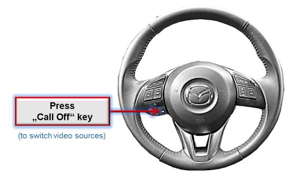
To switch the video sources the vehicle's infotainment button at the steering wheel can be used.
