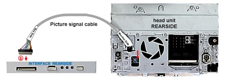
Connect the picture signal cable's female 20pin connector "BOX SIDE" to the 20pin connector of the video interface, with its contacting side in the UP position.
