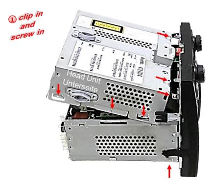
(1) Clip in the head unit housing's mounting locations and again fix the parts to the monitor by using the 4 original Torx screws.
