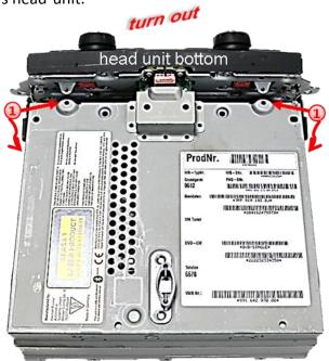
1 Turn out both Torx screws of the head unit's bottom part of the head unit (red arrows) and both Torx screws at the upper part of the head unit.
