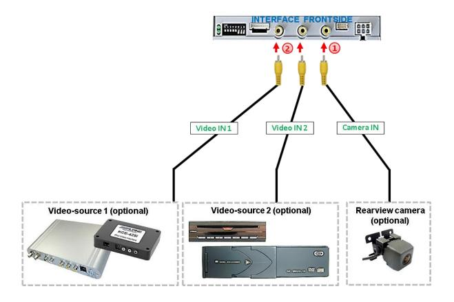
1 Connect the rear-view camera's RCA to the female RCA "Camera IN" of the video cable.
