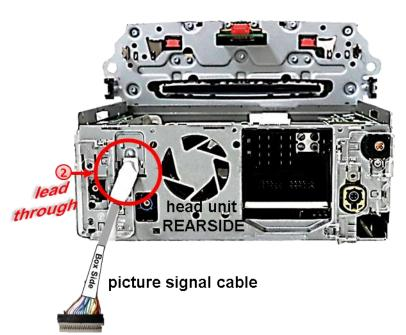
① Connect the picture signal cable's female 20pin **c**onnector **"MONITOR SIDE"** with its contacting side in down position to the 20pin connector of the installed daughter PCB inside the head unit.
