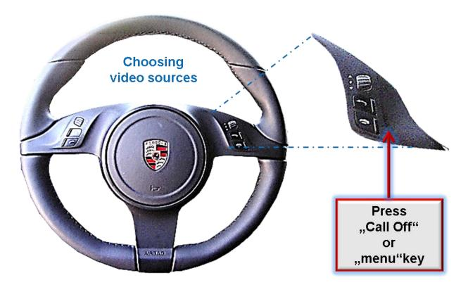
To switch the video sources the vehicle's **Call off button** or **menu button** can be used.
