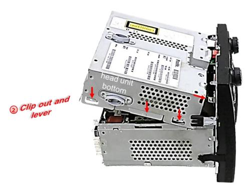
2 Clip out and lever the fixing points of the head unit's upper and lower housing parts (red arrows) all around the housing and carefully separate both parts.
