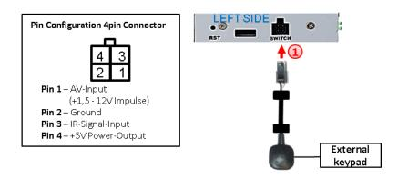
1 Connect the keypad's female 4pin connector to the male 4pin connector of the video-interface.
