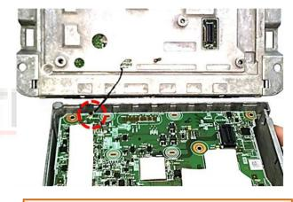
Carefully separate the rear-side from the monitor.
