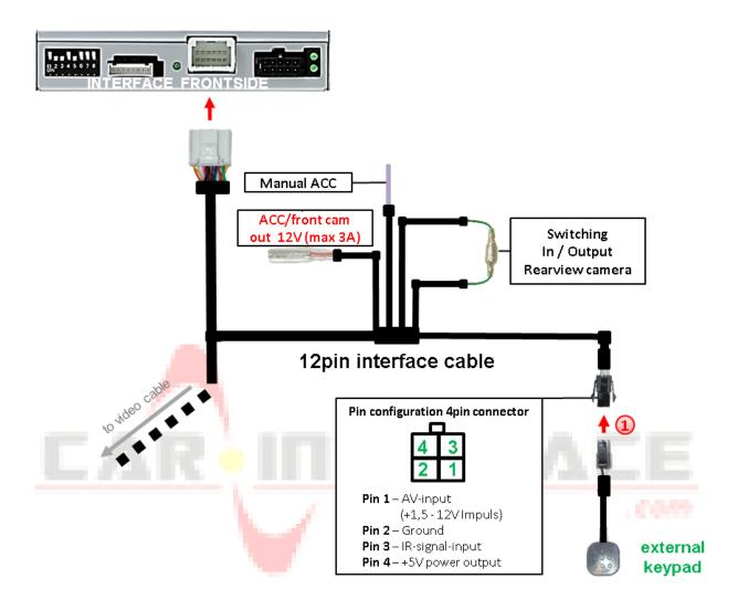
1 Connect the keypad's female 4pin connector to the 12pin interface cable's male 4pin connector.
