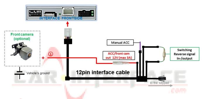
The red power supply output ACC/front cam out 12V (max 3A) can be used to power a front camera. If Dip 1 is set to ON (black 8 dips), the power supply output gives +12V (max 3A) when reverse gear is engaged incl. 10 seconds delay after reverse gear is disengaged.
