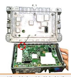
Reconnect the original coaxial cable back to the main PCB board as shown above.
