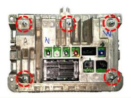
Screw out the 5 screws at the rear-side of the monitor housing.
