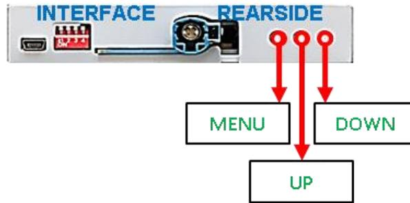
The picture settings are adjustable by the 3 push-buttons of the daughter PCB's menu keypad. Press the 1. button to open the OSD settings menu or to switch to the next menu item. By pressing the other both push buttons the selected value will be changed. To avoid accidental changes during or after the installation, we recommend to disconnect the keypad from the pushbutton cable after the adjustments are done. Adjustments have to be done, while the selected input is visible on the monitor.
