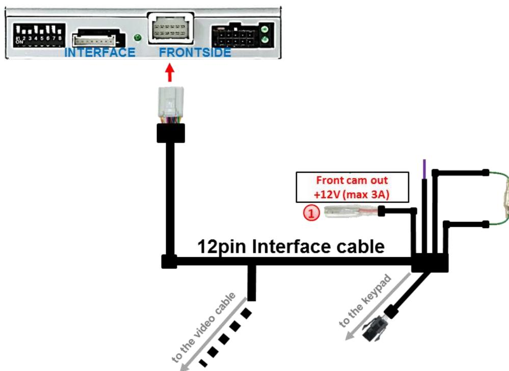
① The red power supply output **Front cam out +12V (max 3A)** can be used to power a front cam with dip switch 1 (of the black 8 dips) to ON.
