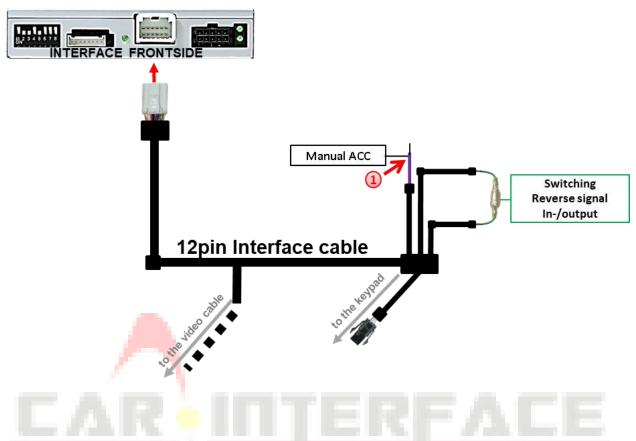
1 If, after connecting the PNP harness, no interface LED lightens up while the ignition is turned on, the purple coloured wire Manual ACC of the 12pin interface cable has to be connected additionately to ACC or S-contact terminal 86s +12V (e.g. glove compartment illumination).
