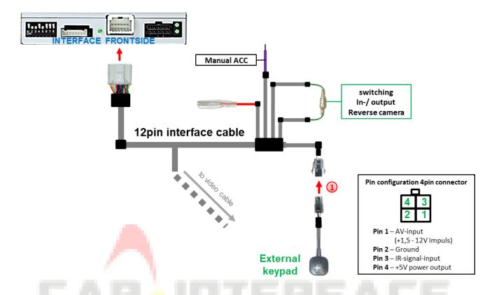
Connect the female 4pin connector of the keypad to the male 4pin connector of the 12pin interface cable.
