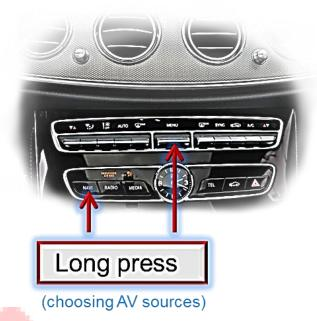
To switch the interface's activated video sources, the factory infotainment's menu or Navi buttons can be used.
