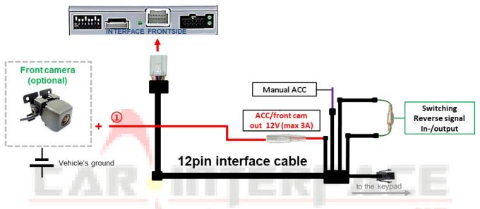
The red power supply output ACC/front cam out 12V (max 3A) can be used to power a front camera. If Dip 1 is set to ON (of the black 8 dips), the power supply output gives +12V (max 3A) when reverse gear is engaged plus 10 seconds delay after reverse gear is disengaged.
