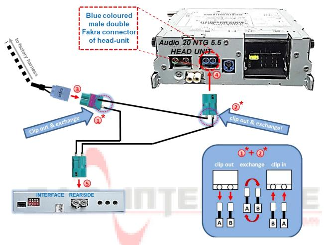
Unlock the picture signal cable's **green-coloured** male double Fakra connector's locking mechanism, clip out both cables to exchange them (see the blue diagram), clip in the exchanged cables and again lock the connectors locking mechanism.
