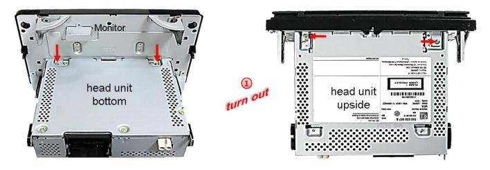
Turn out both screws at the **outer** side of the top part of the head unit (red arrows) and both screws at the bottom part of the head unit (red arrows). Remove the head unit from the monitor and lay it aside.
