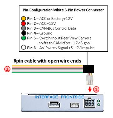
Connect the female 6pin connector of the 6pin cable to the 6pin connector of the video interface.
