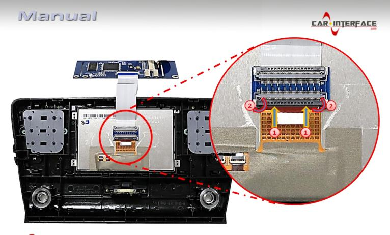
Carefully lead the monitor's brown colored 50pin ribbon cable into the preassembled ribbon cable merger of the daughter PCB's 50pin ribbon cable "PNL-OUT". Make sure that the connector pins are faced to the merger's platinum.
