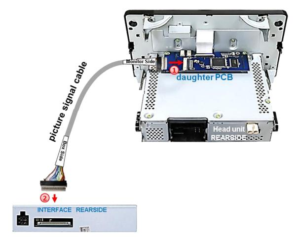
If not preassembled, connect the beige colored male 20pin connector (Monitor Side) of the 20pin picture signal cable to the female 20pin connector of the daughter PCB.
