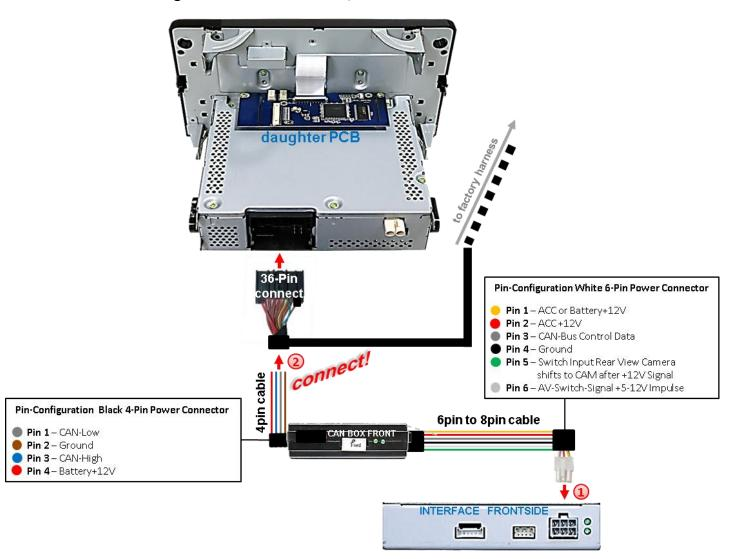
Connect the white female 6pin connector of the 6pin to 8pin cable to the male 6pin connector of the video interface.
