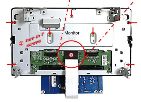
Fix the monitor's rear metal sheet by using the 7 screws.
