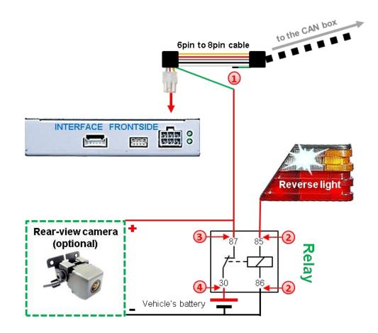
Out the green cable of the 6pin to 8pin cable close to the black 8pin connector and isolate the shorter end of the green cable near to the 8pin connector (CAN-box side).
