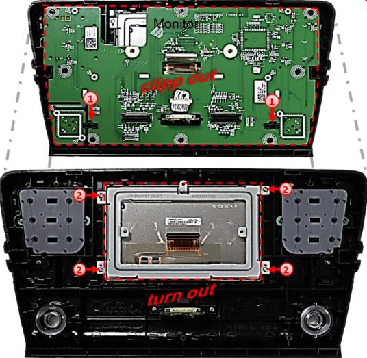
Clipp out the monitor's mainboard from the monitor's front housing and put it aside for setting free the monitor panel's metal frame and the 50pin ribbon cable for its connection to the daughter PCB.
