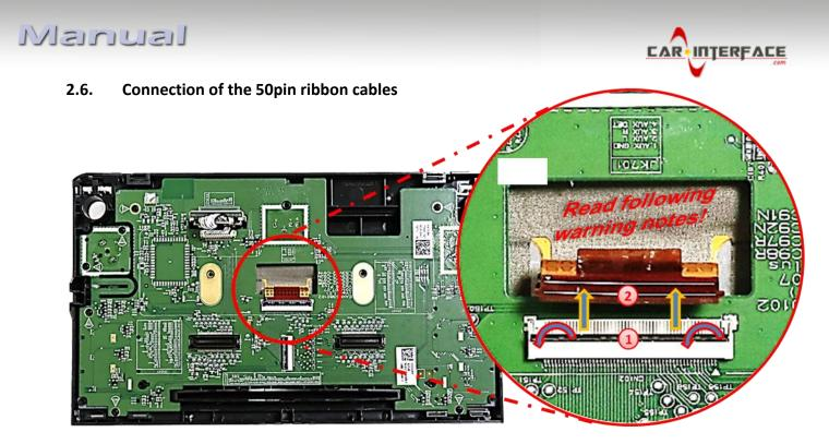
Fold upwards the black hinge of the factory ribbon cable base to unlock the original brown colored 50pin ribbon cable of the factory PCB.
