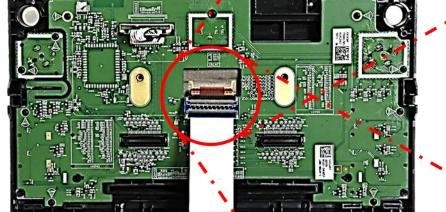
To avoid any kind of vibration-caused short circuits after the connection, it's necessary to isolate both sides of the merger with some kind of smooth issue tape as shown in the picture beside.
