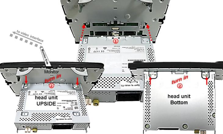
Reassemble the head unit housing to the monitor housing. Take special care for the perfect fitting of both parts and for not to get caught the small white cables of the 12pin connector.
