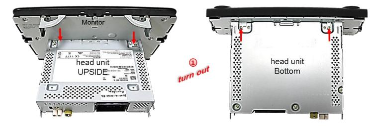
Turn out both screws at the **outer** side of the top part of the head unit (red arrows) and both screws at the bottom part of the head unit (red arrows). Separate the head unit from the monitor and lay it aside.
