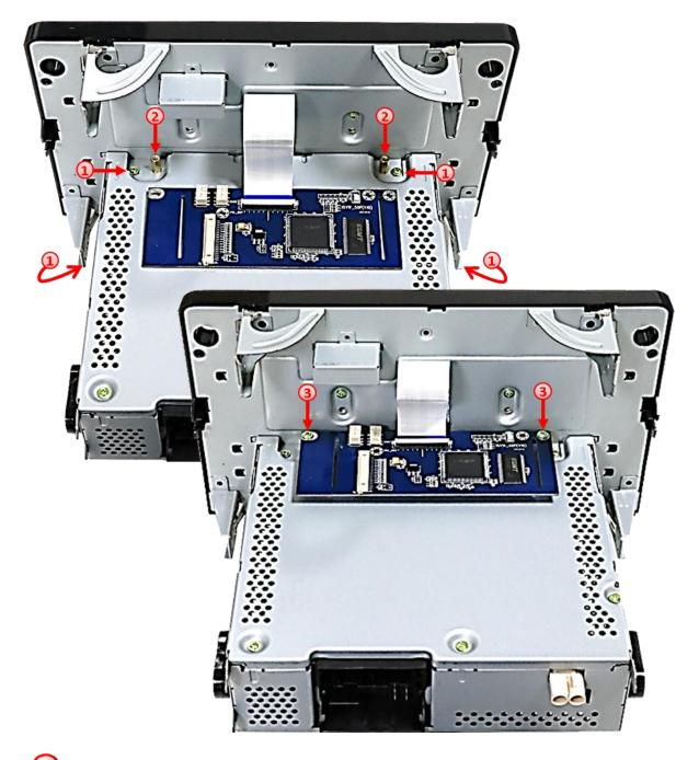
U Carefully, plug the head unit into the monitor again and fix it with the 4 screws on its top and its bottom.
