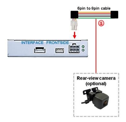
Additionally, the +12V (max. 500mA) power supply for the rear-view camera can be taken from the green wire of the 6pin to 8pin cable.
