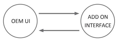
Press and hold "MENU" or "BACK" button on iDrive controller for 3S to switch menu. It will also switch to add on interface automatically after plugging a mobile phone or USB stick.
