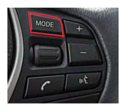
Press and hold "MODE" on steering wheel for 10S will reboot the interface
