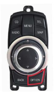
Press and hold "OPTION" for 3S to display front view camera
