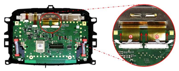
① Open both black locks of the PCB's ribbon cable bases in direction to the arrows and carefully set free the two ribbon cables.
