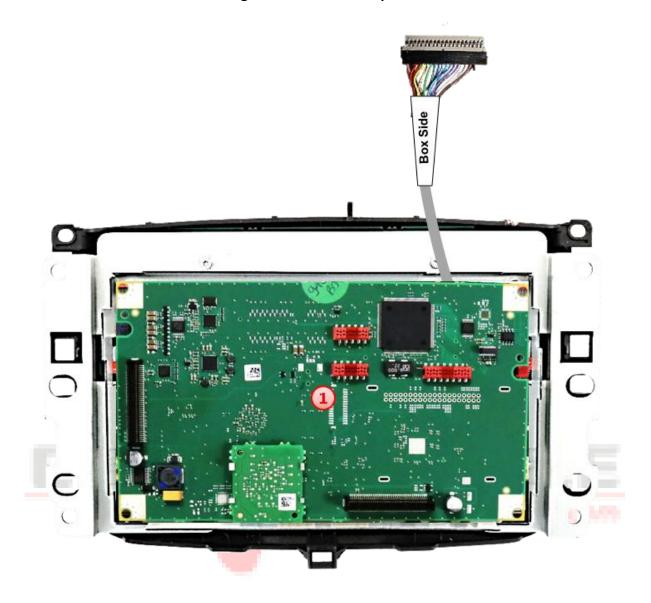
1 Bring the previously set aside original PCB in position with its 4 screw holes to the thread sockets of the exchange metal plate-2 and restore the connection of the plug contacts.
