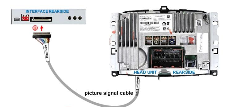
1 Connect the picture signal cable's beige coloured female 20pin connector, which is lead out from the head unit, to the male 20pin connector of the video-interface.
