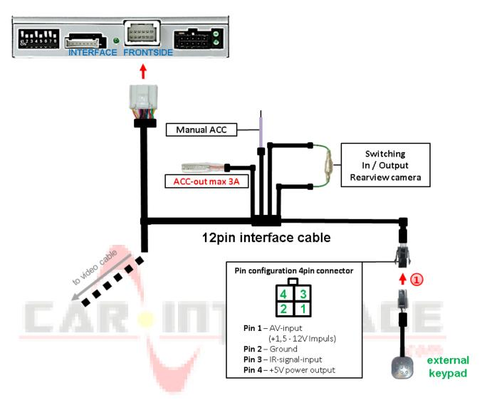
Onnect the keypad's female 4pin connector to the video-interface's male 4pin connector.
