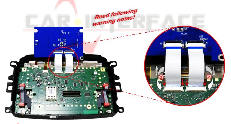
2 Bring the daughter PCB in position and connect it's preconnected ribbon cables "IN" to the previously become free ribbon cable bases of the original PCB. Carefully fix the ribbon cables by pushing the locks in direction of the arrows as shown in the illustration.
