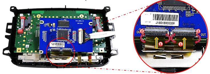
Carefully lead both mainboard's previously become free gold coloured ribbon cables into the daughter PCB's ribbon cable bases "OUT".
