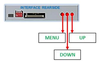
The picture settings are adjustable by the 3 push-buttons of the daughjter PCB's menu keypad. Press the 1. button to open the OSD settings menu or to switch to the next menu item. By pressing the other both push buttons the selected value will be changed. To avoid accidental changes during or after the installation, we recommend to disconnect the keypad from the pushbutton cable after the adjustments are done. Adjustments have to be done, while the selected input is visible on the monitor.
