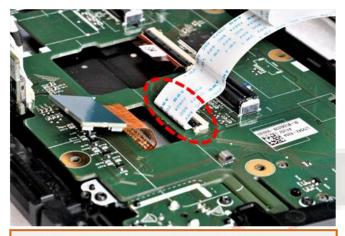
Clip the second enclosed ribbon cable to the previously become free ribbon cable base of the monitor board with the contacts facing upwards.
