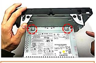
Screw out the two fixing screws at the head unit's upper side.
