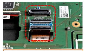
Unclip the copper-coloured factory ribbon cable from the ribbon cable base of the monitor board and clip it to the ribbon cable base of the enclosed ribbon cable merger (pre-assembled).
