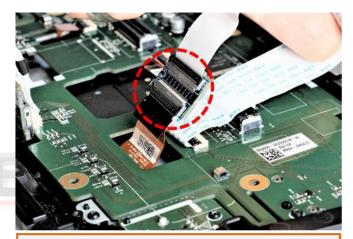
After connecting both ribbon cables, protect ribbon cable merger and ribbon cables from short circuits or cable damage with tape when leading them out before reassembling the monitor panel. See also Fig. 5 and 6
