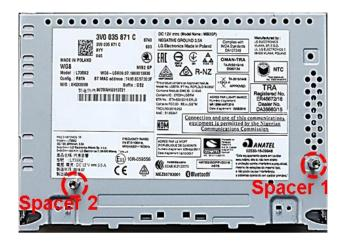
Mount the second spacer to the head unit housing and fix it on the opposite, if necessary.
