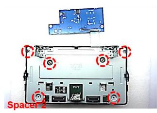
Close the monitor housing with the metal bracket and fix it with 4 of the original screws at the edges. The 2 enclosed spacers have to be screwed in the 2 free middle holes for the daughter PCB's fixing.
