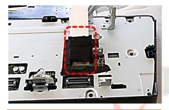
Before leading out the ribbon cables, the ribbon cable merger and the ribbon cables have also to be protected with tape to prevent cable damage and short circuits.
