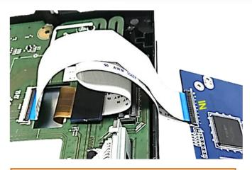
Connect the daughter PCB's ribbon cable "IN" to the previously become free monitor PCB's ribbon cable base.
