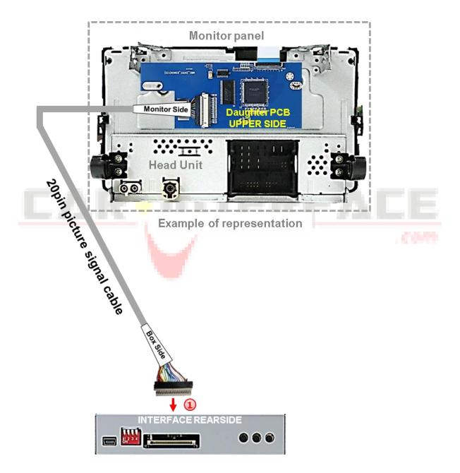
Connect the female 20pin connector of the daughter PCB's pre-connected 20pin picture signal cable to the video interface's male 20pin connector.
