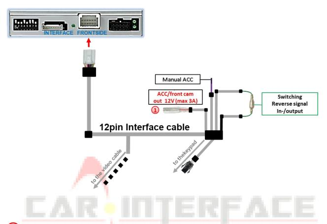
The red power supply output ACC/front cam out 12V (max 3A) can be used to power an external source and has a different assignment, depending on the position of dip switch 1 (of 8 dips):
