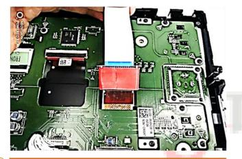
Bevor placing and outleading the daughter PCB's ribbon cables, the ribbon cable merger has to be isolated to save the system from short circuits.
