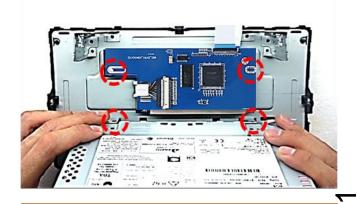
Fix the PCB with 2 screws. Fix the monitor with installed PCB to the head unit with the screws at the upper and the bottom side of the head unit.
