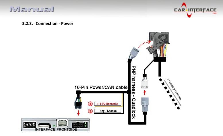
(1) Connect the single yellow wire of the 10pin power/CAN cable to +12V permanent and stabile power supply.
