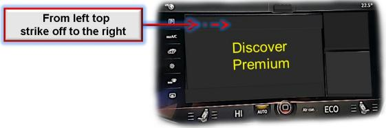
Striking-off from the left top corner to the right of the touch display switches the interface's activated video sources.
