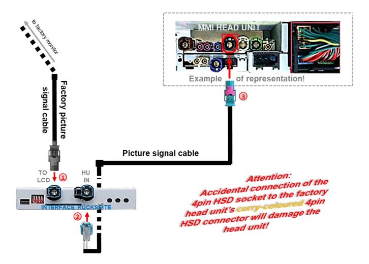
Disconnect the black female HSD connector at the rear-side of the head unit and connect it to the waterblue coloured male HSD connector "TO LCD" of the video interface.
