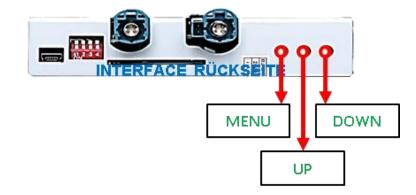
The picture settings are adjustable by the 3 push-buttons at the rear-side of the videointerface. Press the MENU button to open the OSD settings menu or to switch to the next menu item. Press UP and DOWN to change the selected value. The buttons are placed inside in the housing to avoid accidental changes during or after the installation. Picture settings must be done separately for all video inpouts while the corresponding input is selected and visible on the monitor.
