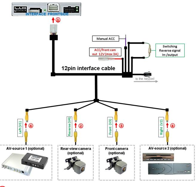
Connect the 12pin interface cable's female 12pin connector to the male 12pin connector of the video-interface.
