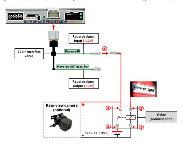
① Disconnect the green cable's preconnected male- and female connectors of the 12pin cable and connect the green input cable "Reverse-IN" to the output connector (87) of the relay.
