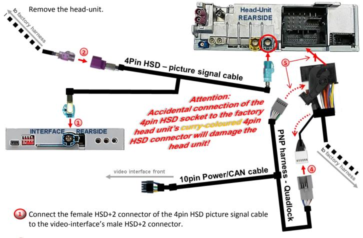
2 Disconnect the female 4pin HSD connector of the vehicle harness from the rear of the head-unit and connect it to the male 4pin HSD connector of the 4pin HSD picture signal cable.
