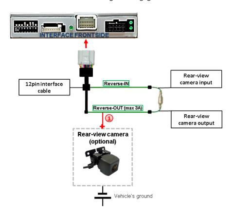
Additionally, the +12V (max. 3A) power supply for the rear-view camera can be taken from the green wire of the 12pin interface cable.
