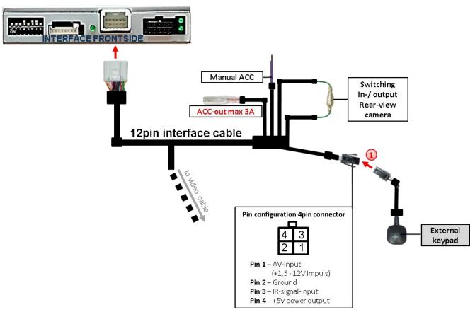
Connect the female 4pin connector of the keypad to the male 4pin connector of the 12pin interface cable.
