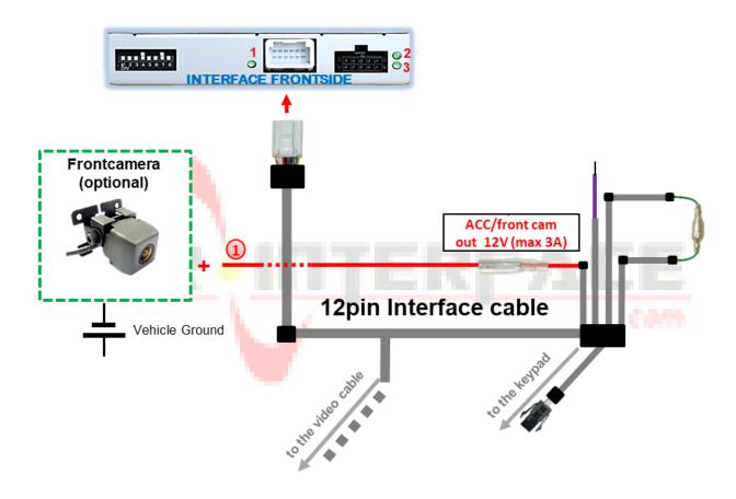
The red power supply output ACC/front cam out 12V (max 3A) can be used to power a front camera. If Dip 1 is set to ON (of the black 8 dips), the power supply output supplies +12V (max 3A) when the reverse gear is engaged and additionally 10 seconds delay after reverse gear is disengaged.
