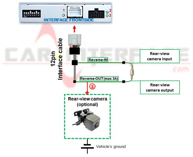
1 The 12 V power supply for the rear-view camera (max 3A) has to be taken from the green wire of the 20pin cable to avoid an unnecessary, permanent power supply to the camera electronic.
