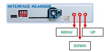
The picture settings can be adjusted by the 3 buttons on the video-interface. Press the MENU button to open the OSD settings menu. To switch to the next menu item, pressing UP and DOWN will change the selected value. The buttons are embedded in the housing to avoid accidental changes during or after installation. The picture settings have to be done separately for AV1 and AV2 while the corresponding input is selected and visible on the monitor.
