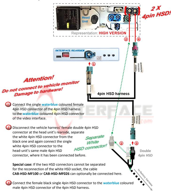
Connect the opposite **waterblue** coloured female 4pin HSD connector of the 4pin HSD harness to the previously become free male 4pin HSD connector of the head-unit.
