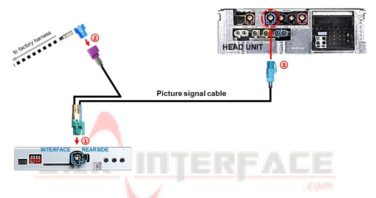
Connect the female waterblue coloured 4+2pin HSD connector of the picture signal cable to the male 4+2pin HSD LVDS connector of the interface-box.
