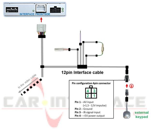
1 Connect the female 4pin connector of the keypad to the male 4pin connector of the 12pin interface cable.
