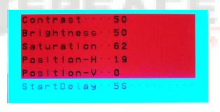
\* Setting only required for errors such as faulty touch function or OEM black image. Note: If a longer start delay is selected, the camera image is delayed accordingly after the vehicle is restarted and the R gear is engaged.
