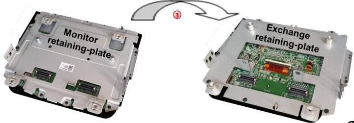
3 Remove the Original monitor retaining plate and replace it with the exchange retaining-plate by using the original screws.
