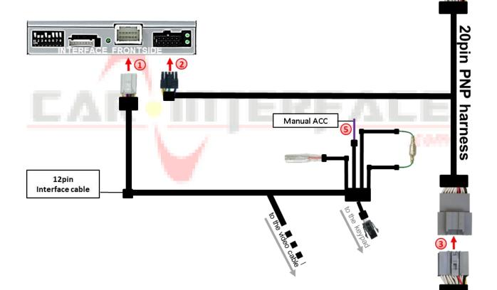
4 Connect the female 20pin connector of the 20pin PNP harness to the male 20pin connector of the head-unit.
