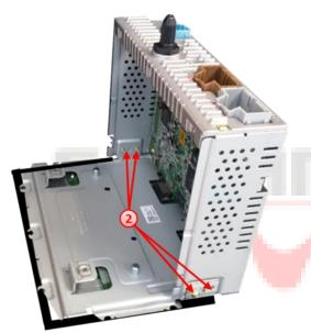
Turn out the 4 screws of the monitor retaining plate.
