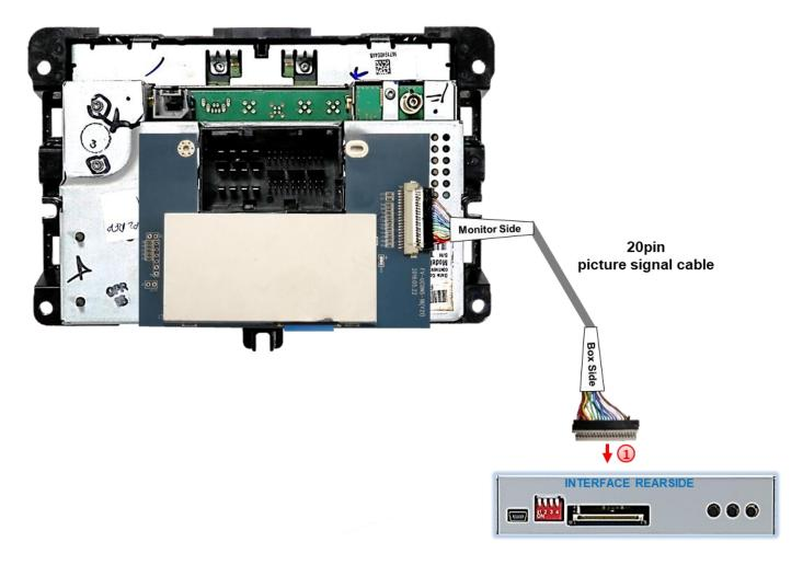
Connect the opposite female 20pin connector of the pre-CONNECTED 20pin picture signal cable to the male 20pin connector of the video interface.
