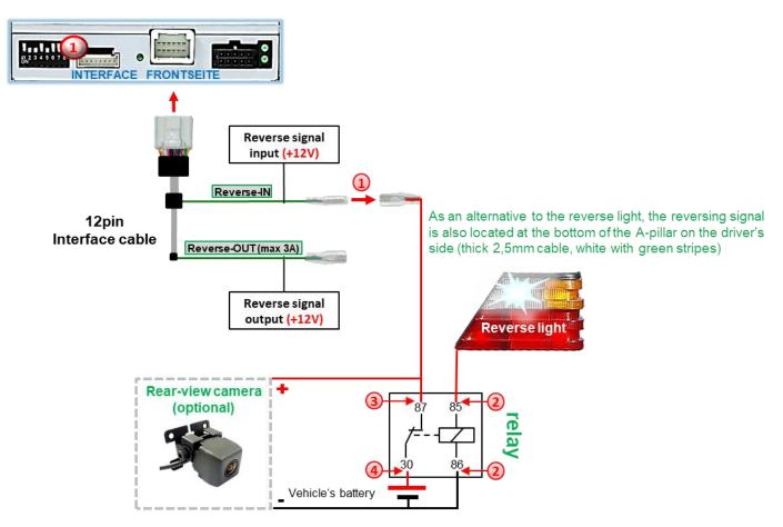
Disconnect the green cable's pre-connected male- and female connectors of the 12pin cable and connect the green input cable **"Reverse-IN"** to the output connector (87) of the relay.
