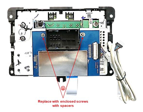
Replace the two original screws, as shown in the picture, with the enclosed longer screws and fix the daughter PCB to the housing by using the enclosed spacers.
