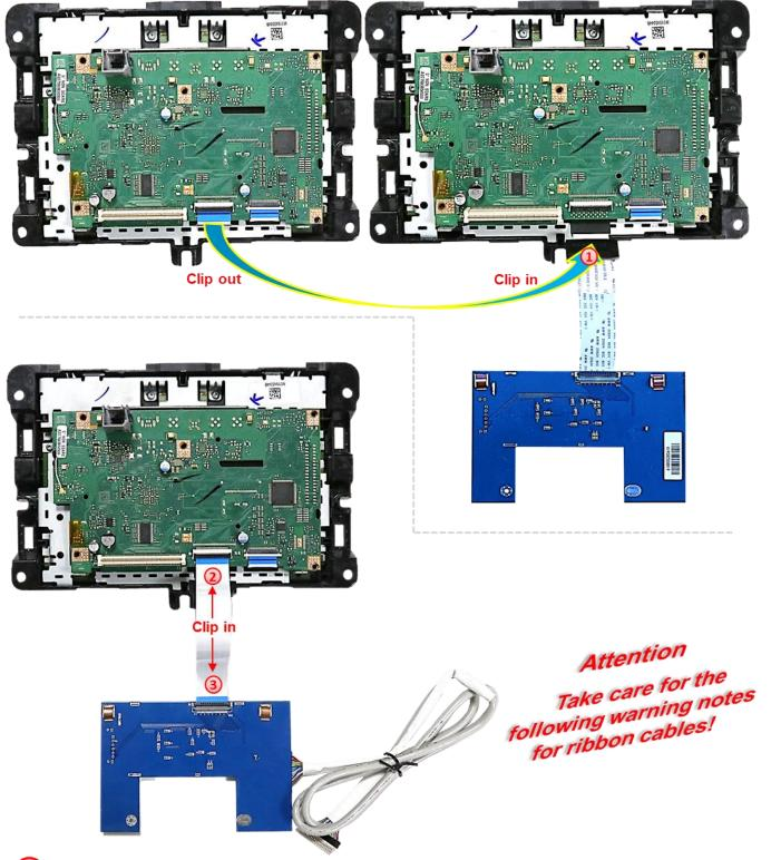
Clip-out and disconnect the monitor board's 40pin ribbon cable, which is coming from the monitor panel, at the ribbon cable base of the monitor board, unplug it and connect it to the pre-connected 40-pin ribbon cable merger of the daughter PCB ribbon cable "OUT" and clip it in.
