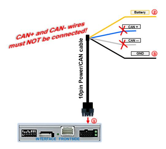
Connect the enclosed 10pin Power / CAN cable's female10pin connector to the male 10pin connector of the video interface.
