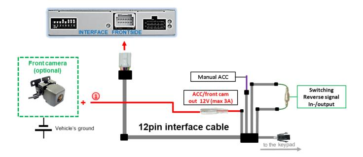
The red power supply output ACC/front cam out 12V (max 3A) can be used to power a front camera. If Dip 1 is set to ON (black 8 dips), the power supply output gives +12V (max 3A) when reverse gear is engaged incl. 10 seconds delay after reverse gear is disengaged.
