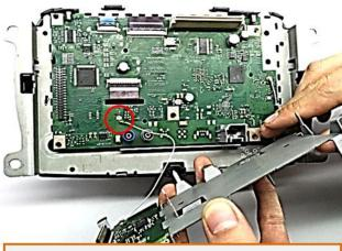
Carefully seperate the metal cover and disconnect the small Coaxial wire connected in between.
