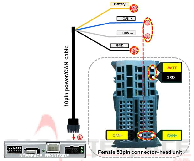
no liability for pin assignment-measurement required!
