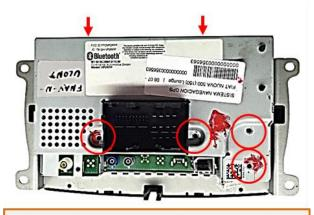
Turn out the screws shown above, to remove the head unit housing's rear cover.
