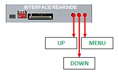
The picture settings are adjustable by the 3 push-buttons of the daughjter PCB's menu keypad. Press the 1. button to open the OSD settings menu or to switch to the next menu item. By pressing the other both push buttons the selected value will be changed. To avoid accidental changes during or after the installation, we recommend to disconnect the keypad from the pushbutton cable after the adjustments are done. Adjustments have to be done, while the selected input is visible on the monitor.
