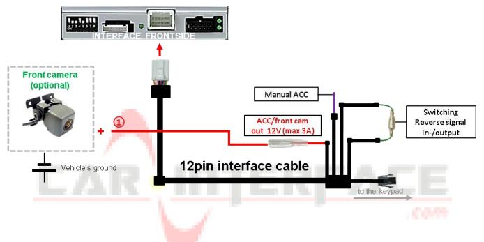
1 The red power supply output ACC/front cam out 12V (max 3A) can be used to power a front camera. If Dip 1 is set to ON (black 8 dips), the power supply output gives +12V (max 3A) when reverse gear is engaged plus 10 seconds delay after reverse gear is disengaged.
