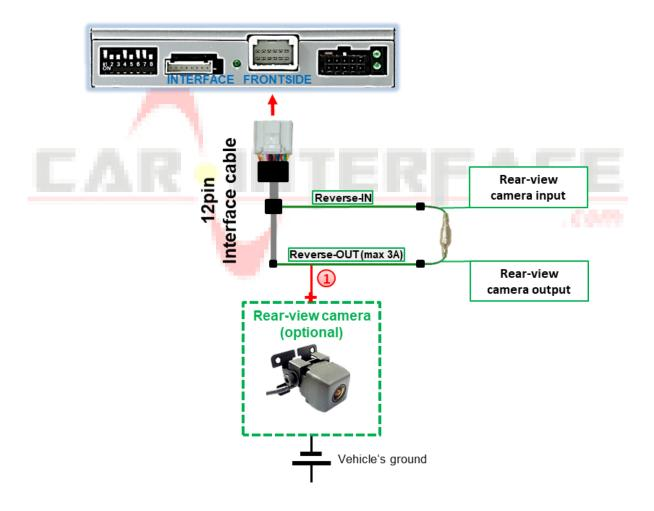
1 The 12 V power supply for the rear-view camera (max 3A) has to be taken from the 12pin interface cabl's green wire "Reverse-OUT" to avoid an unnecessary, permanent power supply to the camera electronic.
