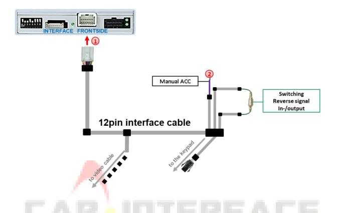
1 If, after connecting the PNP harness, no interface LED lightens up while the ignition is turned on, the purple-coloured wire Manual ACC of the 12pin interface cable has to be connected additionally to ACC or S-contact terminal 86s +12V (e.g. glove compartment illumination).
