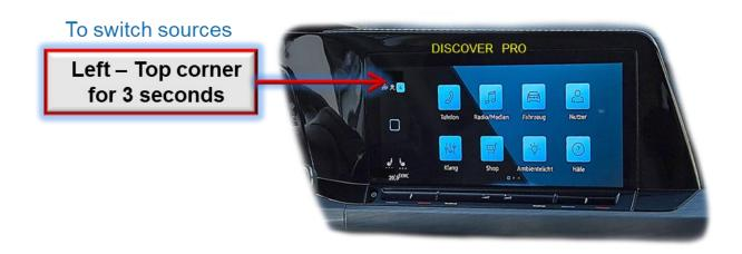
A long press in the touch display's left upper edge switches the interface's activated video sources.
