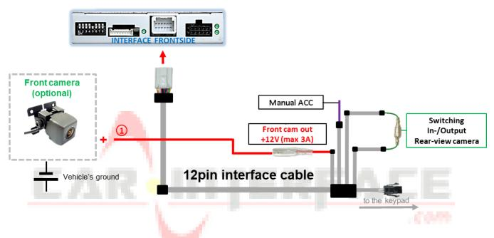
1 The red power supply output ACC/front cam out 12V (max 3A) can be used to power a front camera. If Dip 1 is set to ON (black 8 dips), the power supply output gives +12V (max 3A) when reverse gear is engaged ...
