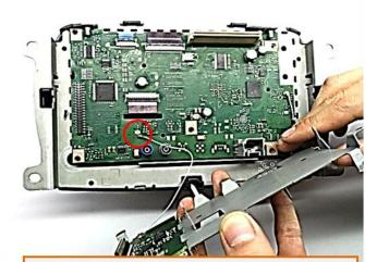
Carefully seperate the metal cover and disconnect the small Coaxial wire connected in between.
