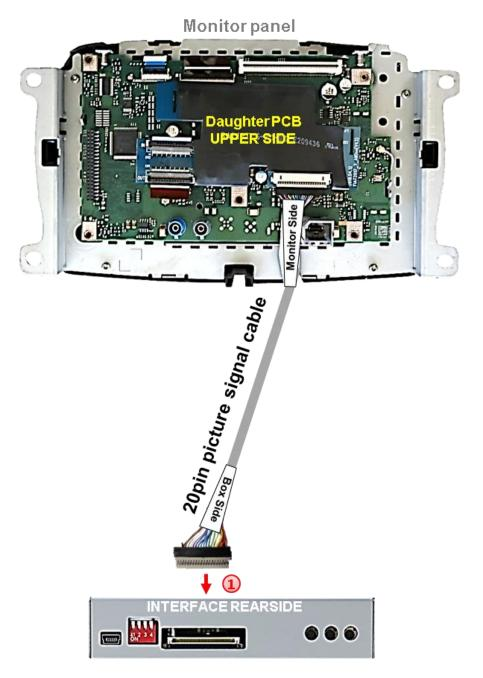
Connect the female 20pin connector "Box Side" of the daughter PCB's pre-connected 20pin picture signal cable to the video interface's male 20pin connector.
