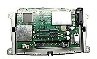
Carefully separate the original PCB from the system. Make sure not to damage the connector.
