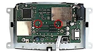
Reinstall the original mainboard and fix it with the original screws
