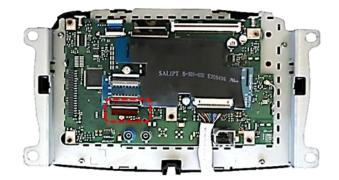
Connect the preveously disconnected 40pin ribbon cable to the 40pin ribbon cable base of the daughter PCB 2.
